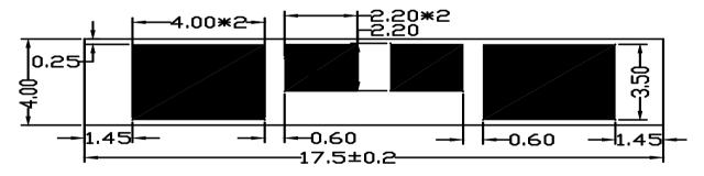
Thickness of the PCB:  $0.60 \pm 0.10$ mm
