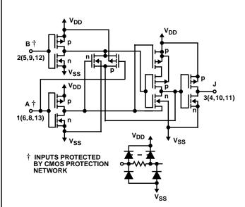
FIGURE 1. SCHEMATIC DIAGRAM FOR CD4070B (1 OF 4 IDENTICAL GATES)
