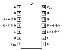
CD4077B (PDIP, CERDIP, SOIC) TOP VIEW
