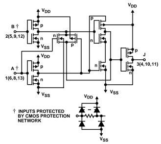
FIGURE 2. SCHEMATIC DIAGRAM FOR CD4077B (1 OF 4 IDENTICAL GATES)
