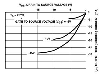
FIGURE 5. TYPICAL OUTPUT HIGH (SOURCE) CURRENT CHARACTERISTICS
