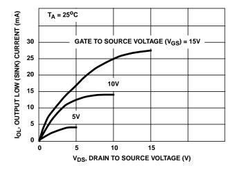
FIGURE 3. TYPICAL OUTPUT LOW (SINK) CURRENT CHARACTERISTICS
