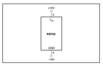
FIGURE 1. Burn-In Circuit.
